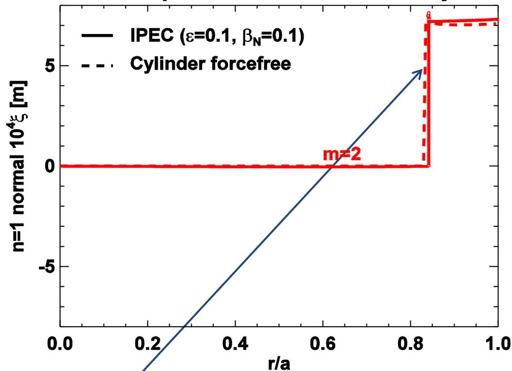
Large radial derivative of displacement associated with large localized current at  $q = 2$  rational surface.
