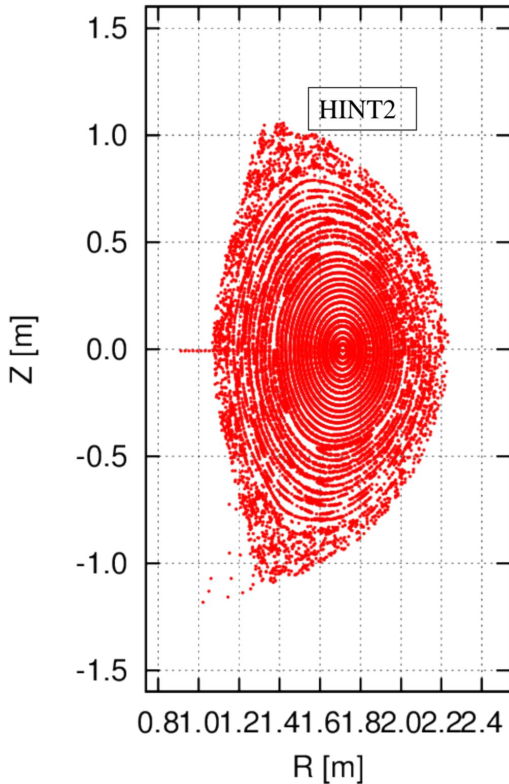
Nonlinear calculations that do not assume good flux surfaces (HINT2, nonlinear M3D-C1 and PIES) find stochasticity in an outer region of the plasma .
