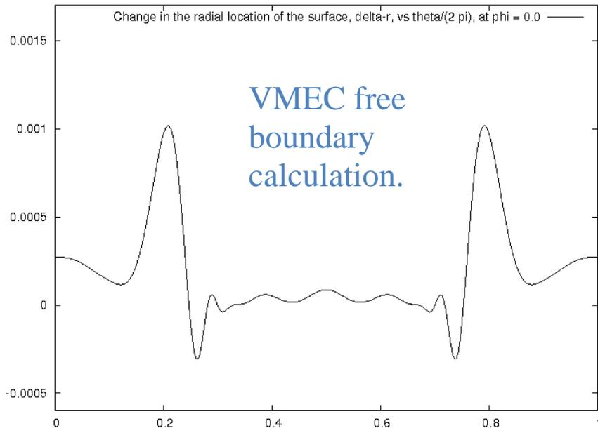
*Amplitude of radial flux surface displacement vs.  $\theta / (2\pi)$  (poloidal angle) for  $q = 8.5/3$  flux surface.*
