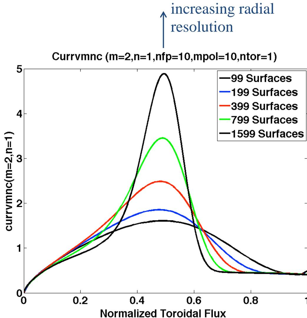
of corresponding  $n = 1, m = 2$  component of current density finds at localized current not all resolved in VMEC calculation. (S. Lazerson)
