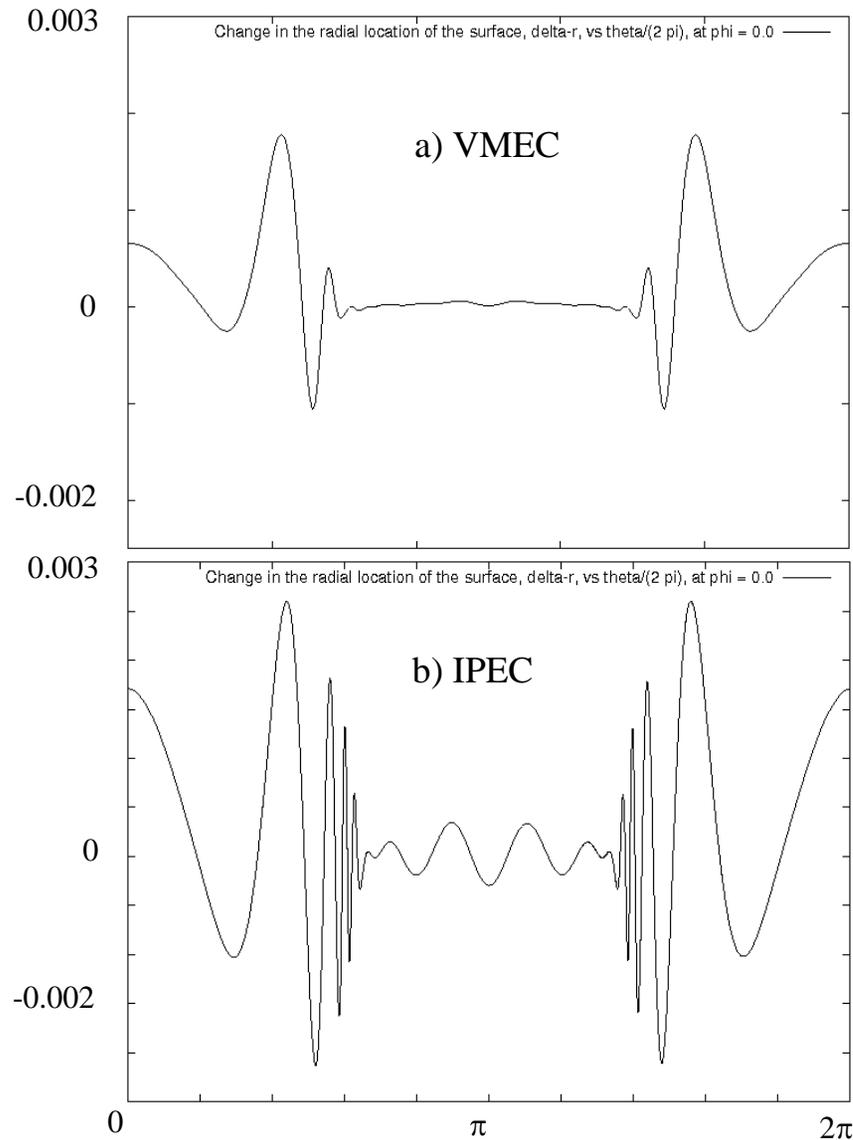
*Comparison of the radial perturbation as a function of poloidal angle for the  $q=13.5/3$  surface as calculated by VMEC and IPEC.*
