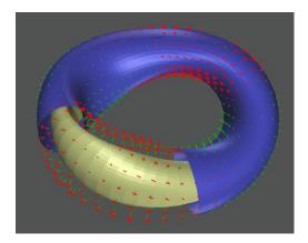
A simple set of circular electromagnets, shown on left. The shaping magnetic field is produced by an array of permanent magnets. Each magnet creates a dipole field, which is represented by an arrow. The total magnetic field created is designed for optimal plasma confinement.
