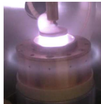
Laboratory test of a liquid-metal cathode. (Photo courtesy of General Electric)
